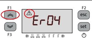
Repair the fault before performing the reset.
